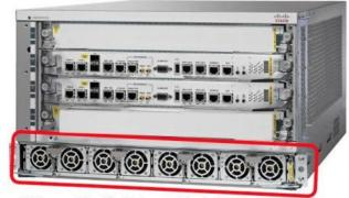
1 Power Shelf, 4 Power Modules 2,1 KW DC/ 3,0 KW AC supplies
